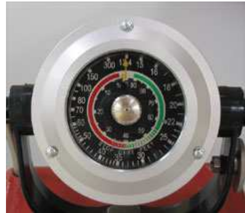
A Tapley meter should be used to MoT test DAF brakes
